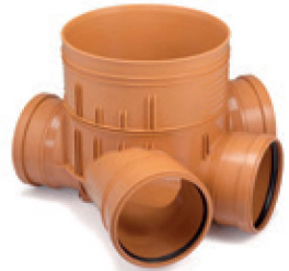
K35P16ZB dedicated for \varnothing 160 pipes K35P20ZB dedicated for \varnothing 200 pipes The chamber base with a backwater valve for corrugated riser pipe \varnothing 315 (external diameter of riser pipe \varnothing 355) K35P16 dedicated for \varnothing 160 pipes K35P20 dedicated for \varnothing 200 pipes Straight base, for corrugated riser pipe \varnothing 315 (external diameter of riser pipe \varnothing 355) K35Z16 dedicated for \varnothing 160 pipes K35Z20 dedicated for \varnothing 200 pipes Collection base – 3 inlet, for corrugated riser pipe \varnothing 315 (external diameter of riser pipe \varnothing 355) K35Z16B dedicated for \varnothing 160 K35Z20B dedicated for \varnothing 200 Collection base – 3 inlet, for corrugated riser pipe \varnothing 315 (external diameter of riser pipe \varnothing 355)
