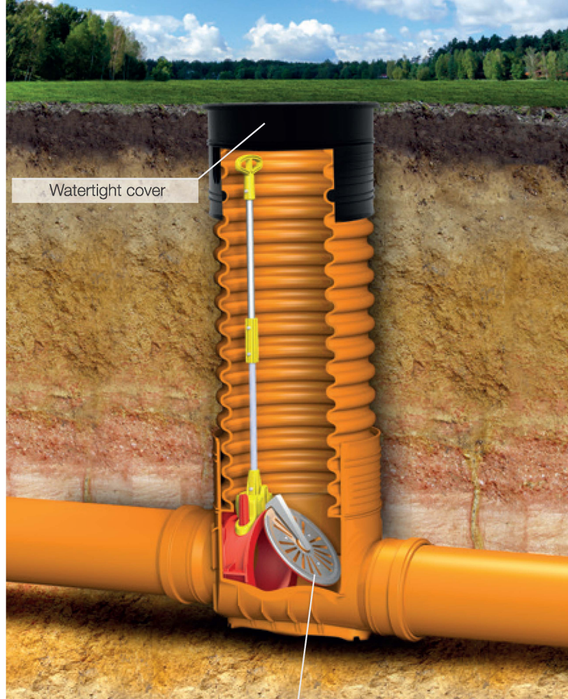
Chamber base with a backwater valve
